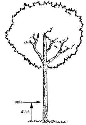
Figure 2-3. Tree Diameter at Breast Height Measurement
